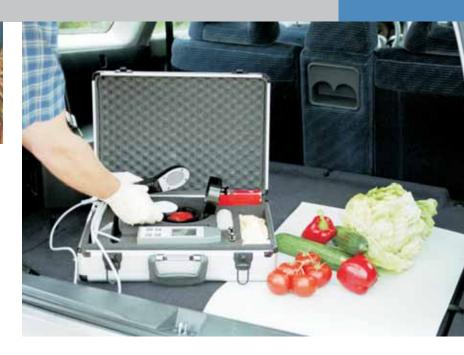
The portable measuring equipment FH 40 LAB-1/ FH 40 G will strongly reduce the loss of time in cases of an emergency involving radioactive contaminations. It is an easy-to-handle mobile radiation laboratory configured specifically for on-site operation. In addition to offering a high degree of mobility, the FH 40 Lab-1 offers advantages in the reproducible sample geometry and comparability of measurements.
